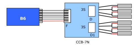
2. Balance three 2S battery pack simultaneously
