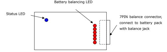
There is one balance connector on the right of CY – B6. For CY – B6. You should assure the connection in accordance with CONNECTION DIAGRAM.
